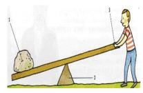
Palanca means lever. Why would we need a lever. A lever makes it easier to move an object.
